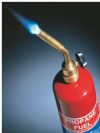
▲ FIGURE 3.8 Propane burning in air. Liquid propane in the tank, C_3H_8 , vaporizes and mixes with air as it escapes through the nozzle. The combustion reaction of C_3H_8 and O_2 produces a blue flame.
